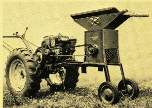
Model 5-N with stabilizer bar attached to garden tractor. Model 5-G with 2 1/2-hp gas engine. Model 5-E with 3/4-hp electric motor.
