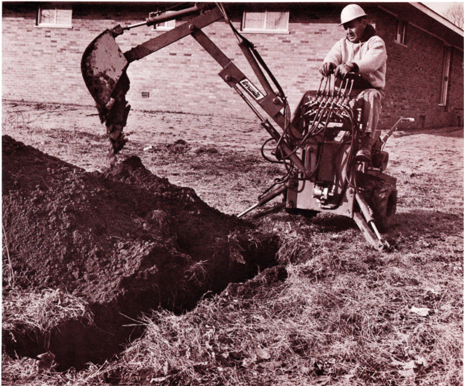
Digs a ditch 16 inches wide, 3 feet deep, and 40 feet long in one hour! Swings vertically 90° . . . 45° to either side.
