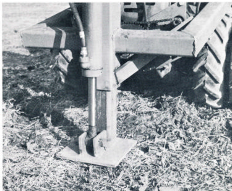
The rear stabilizing leg prevents tipping.
