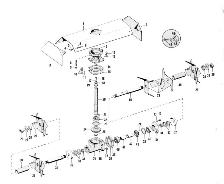
(Covers Models 56, 57, 58-A, and 358. Model Numbers are stamped on the Gear Housing When ordering parts, be sure to refer to the Model Numbers. This list shows parts and prices for the current model, 358 (which is identical to 58-A). Parts for older models are discussed in the "notes", and asterisks ( \* ) are used to show parts which are so discussed.)
