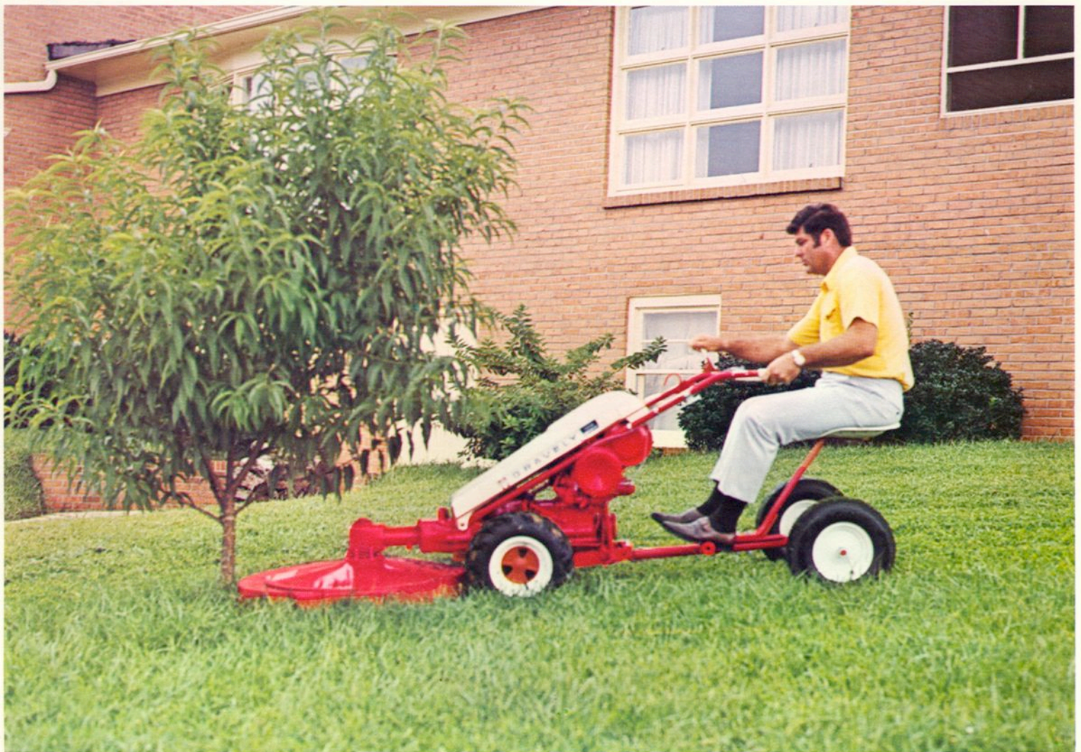
7.6 HP Custom Tractor with 30-Inch Rotary Mower, Optional Chain Guard, and Riding Sulky
