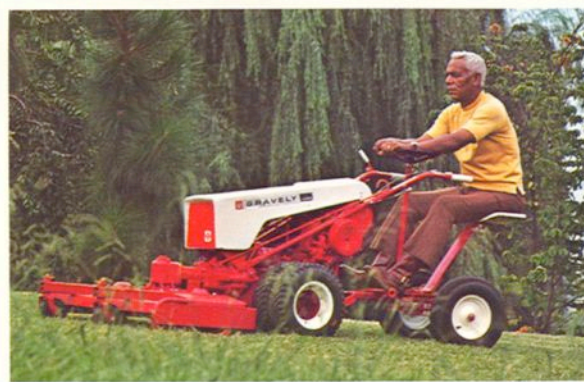
Gravely 7.6 HP Super Convertible Tractor with Steering Sulky, 40-inch Commercial Mower and Dual Wheels
