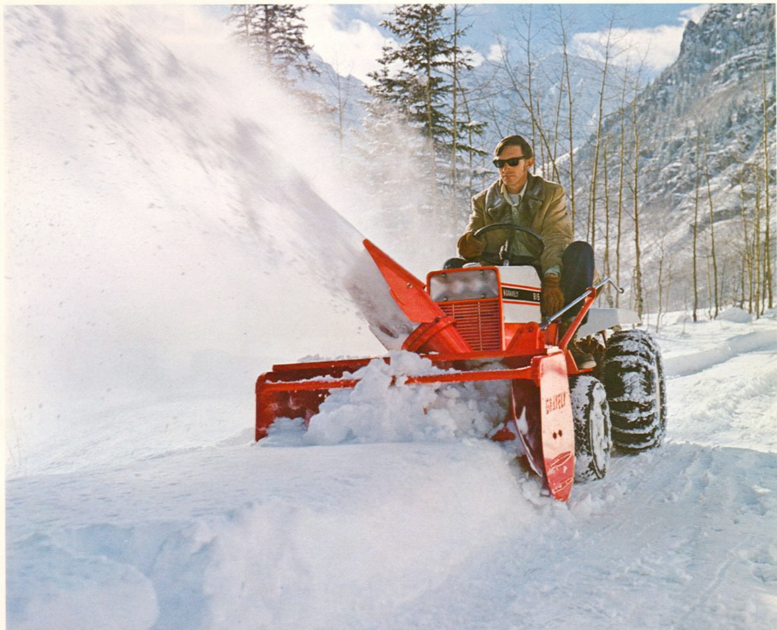
Gravely 816, 16.5 HP Tractor with 44-inch Snowblower
