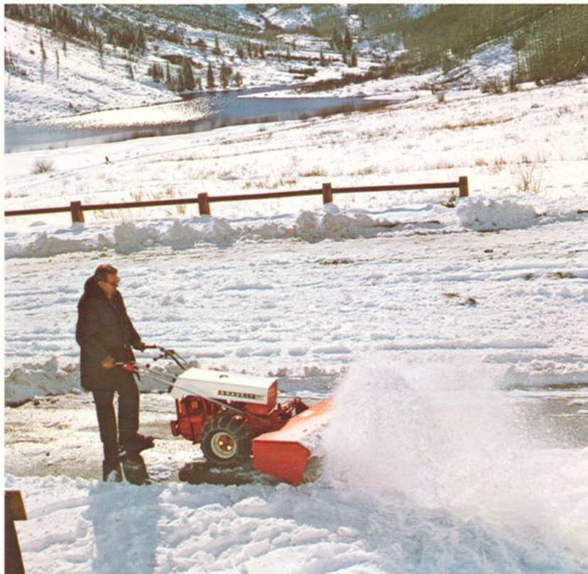
Gravely 12 HP Convertible Tractor with Power Brush, Quick Hitch Kit and Optional Tire Chains
