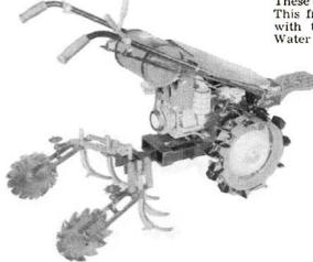
Shown above are five other of the more popular tool arrangements for use on GRAVELY Tractors. Set-up No. 1 shows the Model L Rear Tool Holder with a 12" Furrower attached. This same Furrower may be obtained in any size from 10" to 20". On the Model D better results will be gotten if it is used in front. A 7" shovel steel is available for making smaller openings. All tools are attached to the same steel shanks.
