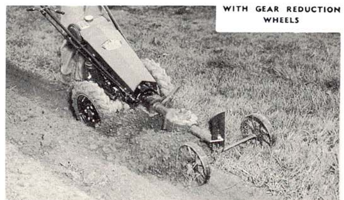
BLADES CUT SIDE AND BOTTOM OF FURROW
