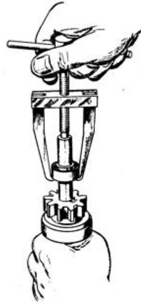
FIGURE 45. MOUNTING OVERRUNNING CLUTCH
