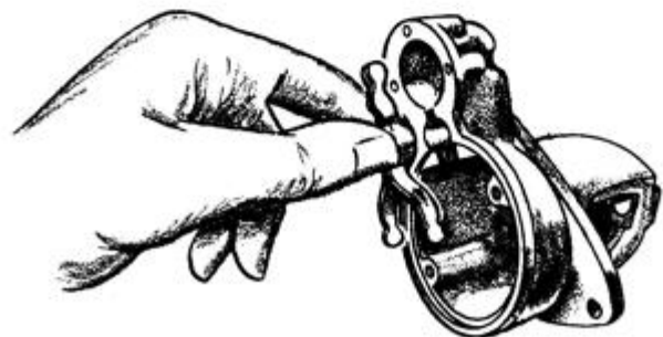
FIGURE 46. INSTALLING SHIFT LEVER
