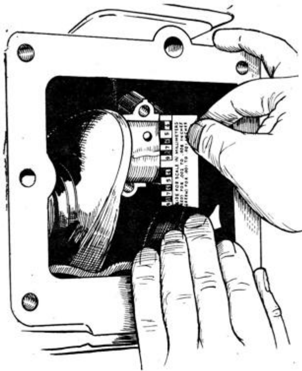
FIGURE 22. MEASURING BEARING CLEARANCE WITH PLASTIGAGE
