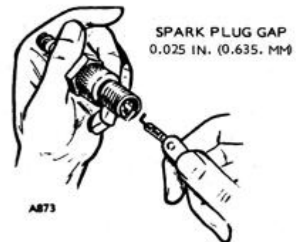
FIGURE 7. CHECKING SPARK PLUG GAP
