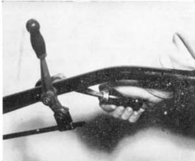
FORWARD: Right hand lever back and down.
