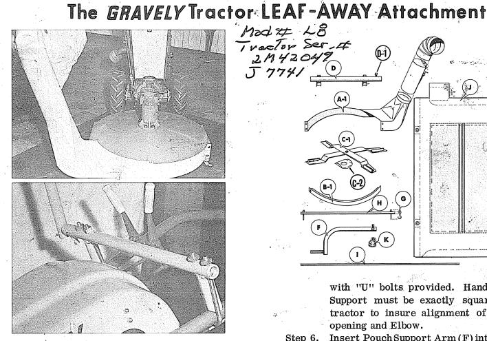
Remove original cutting blade(s) (C). Step 1.
