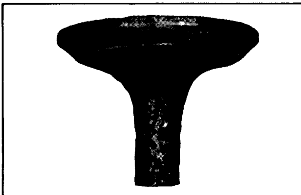
Stem Corrosion: Moisture in fuel or from condensation are the most common causes of valve stem corrosion. Condensation occurs from improper preservation during storage and when engine is repeatedly stopped before it has a chance to reach normal operating temperatures. Replace corroded valves.
