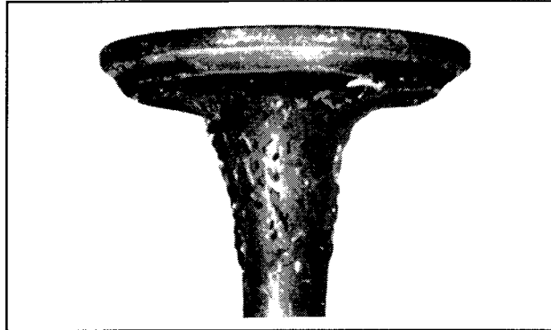
Gum: Gum deposits usually result from using stale gasoline. This condition is often noted in applications where fuel is not drained out of tank during the off season. Gum is a prevalent cause of valve sticking. The cure is to ream the valve guides and clean or replace the valves, depending on their condition.
