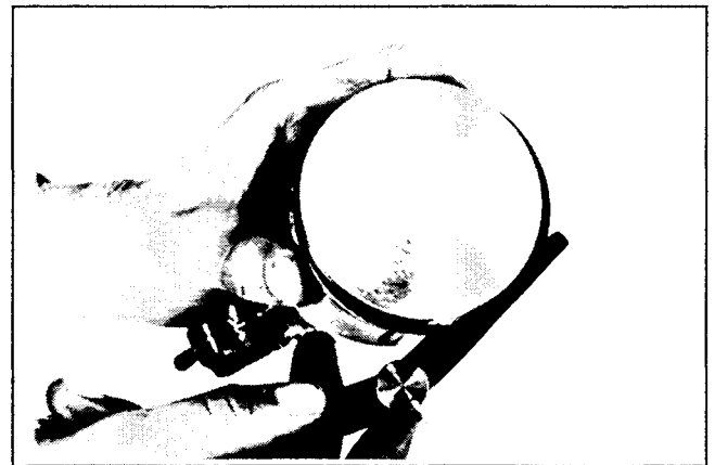
Figure 10-8. Measuring Piston Ring Side Clearance.
