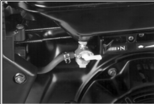
Figure 9-2. Fuel Shut-Off Valve.
