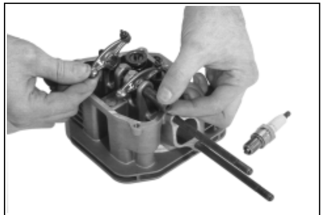
Figure 9-42. CS8.5 (spec. 92xxx), CS10, and CS12 Removing Rocker Arms and Spark Plug.
