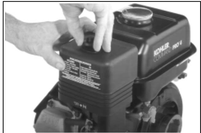
Figure 4-3. Removing Cover Knob Standard.
