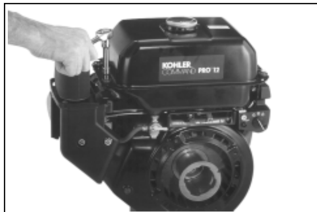
Figure 11-111. Tightening Fuel Tank Mounting Screws.
