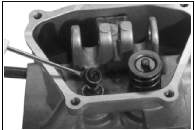
Figure 10-12. Valve Stem Seal.
