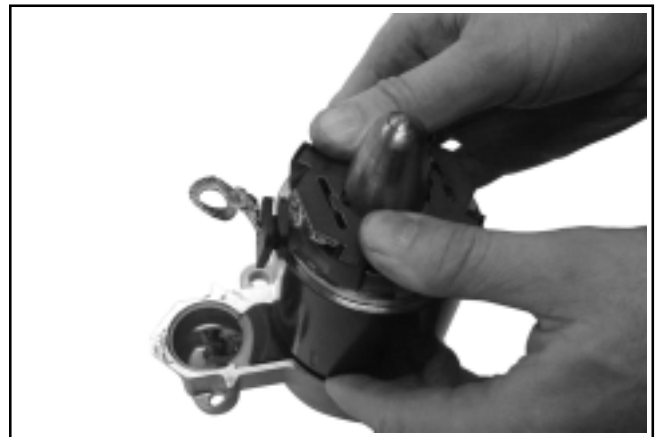
Figure 8-56. Installing Frame with Brush Plate Assembly.
