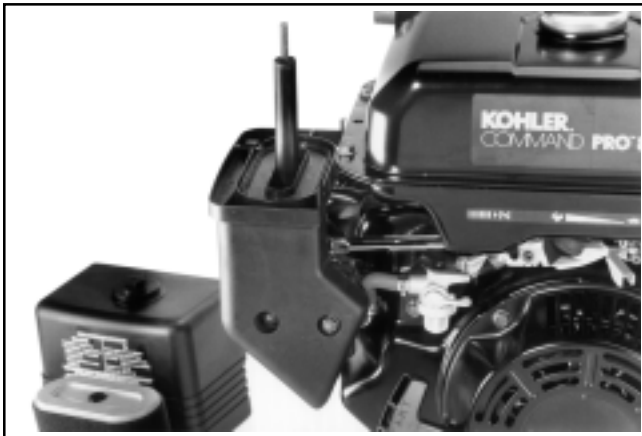
Figure 9-7. CS8.5 (spec. 95xxxx) Air Cleaner Base.
