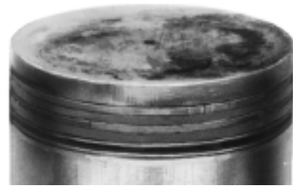
Stuck, Broken Rings
