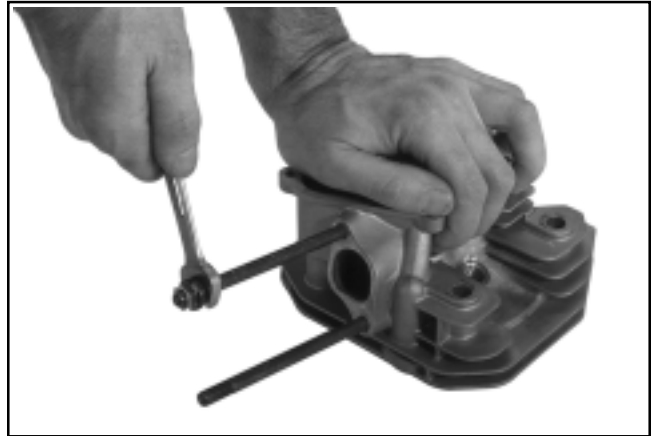
Figure 9-45. Removing Carburetor Mounting Studs.
