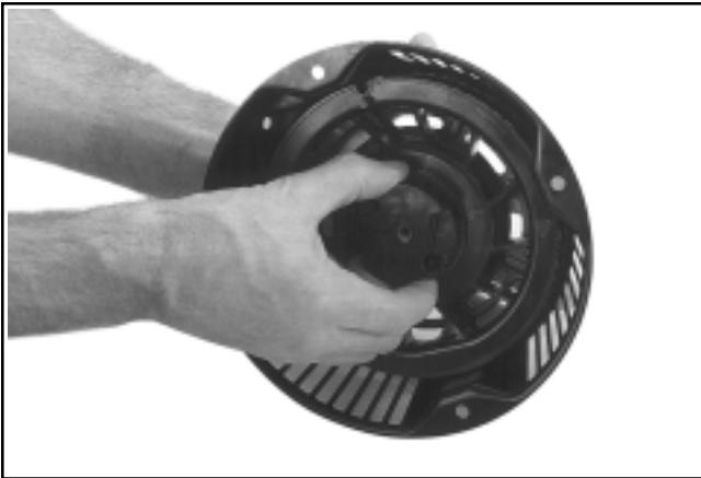
Figure 7-10. Assembling Starter Pulley to Housing.
