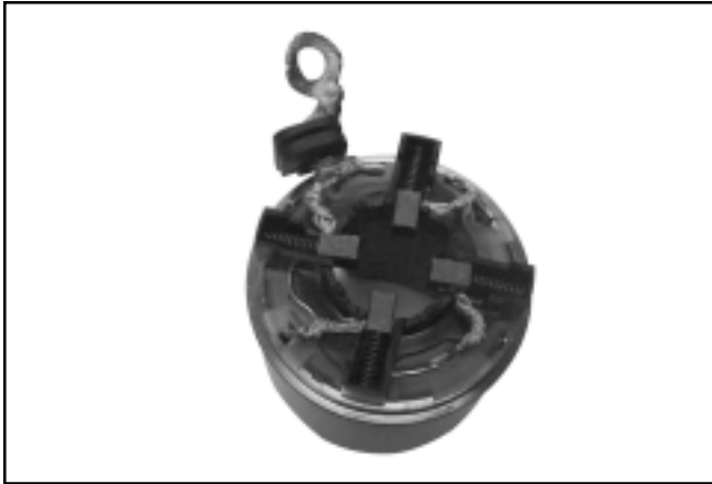
Figure 8-53. Mounting Brush Holder to Frame.
