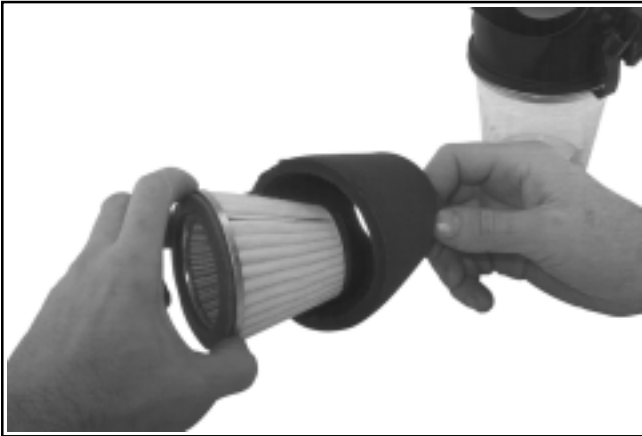
Figure 4-8. Removing Heavy-Duty Precleaner.
