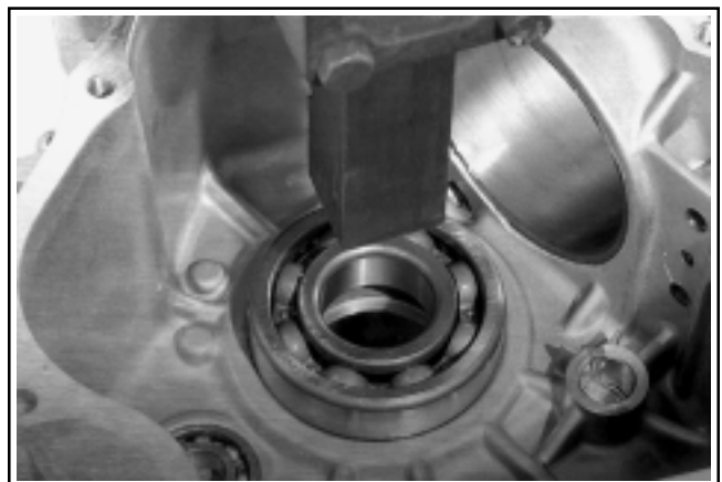
Figure 11-1. Installing Bearings Using a Press.
