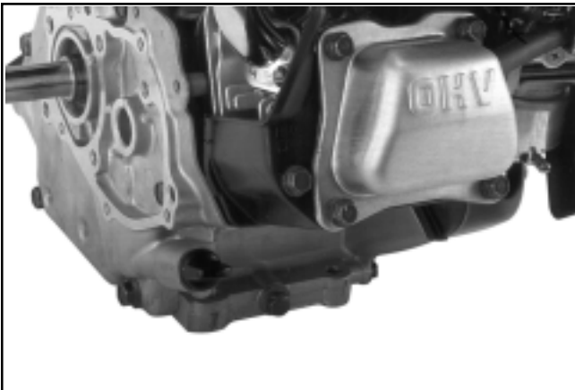
Figure 6-5. CS4, CS6 Left Oil Fill/Level Plug Location.
