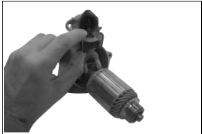
Figure 8-49. Removing Drive Lever and Armature.
