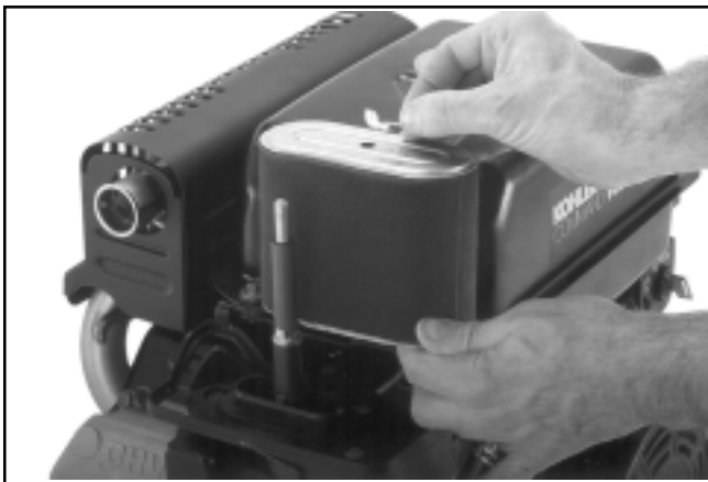
Figure 4-5. Standard Element/Precleaner Assembly.
