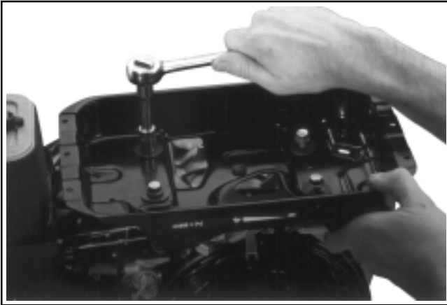
Figure 11-112. CS8.5 (spec. 95xxxx) Installing Fuel Tank Support.
