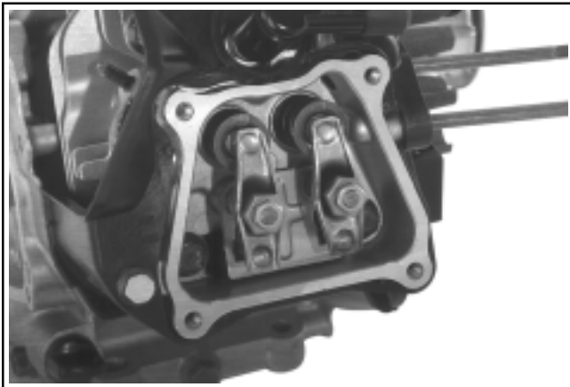
Figure 11-77. CS4, CS6. Cylinder Air Shroud Mounting Bolt Location.
