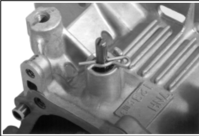
Figure 11-6. CS4, CS6. Installing Hitch Pin.
