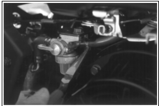
Figure 9-10. Disconnecting Fuel Line on CS8.5 (spec. 95xxxx).
