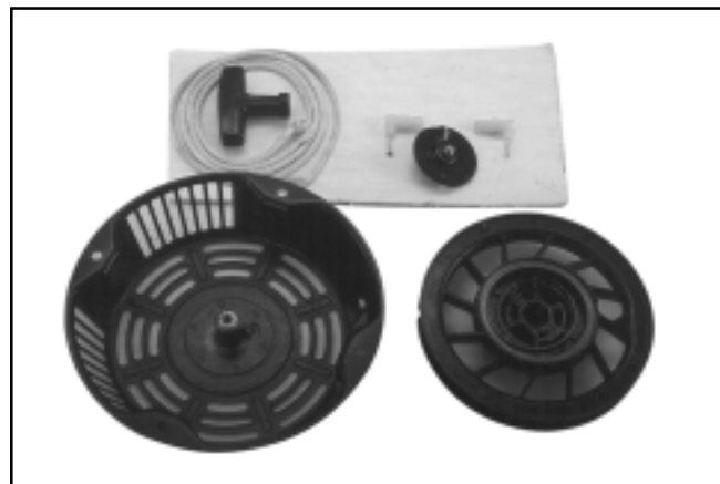
Figure 7-9. Disassembled Retractable Starter.
