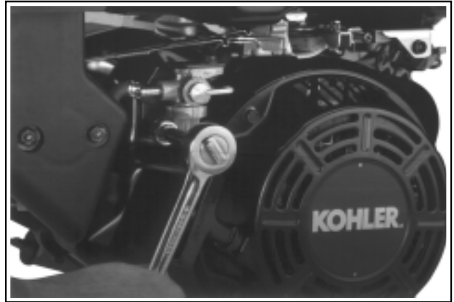
Figure 11-114. CS8.5 (spec. 95xxxx). Mounting Shut-Off Valve.
