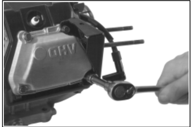
Figure 9-36. Removing Valve Cover Screws on CS8.5 (spec. 92xxxx), CS10, and CS12.
