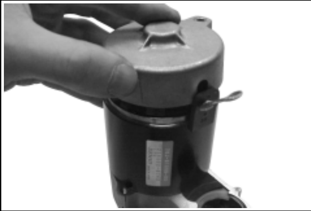
Figure 8-57. Installing End Cap.
