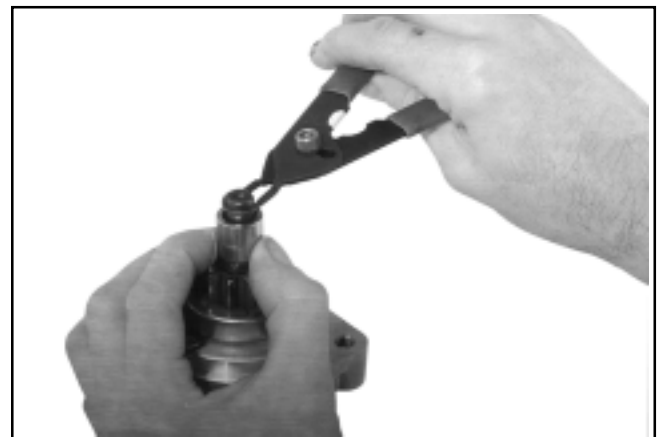
Figure 8-24. Removing Retaining Ring.
