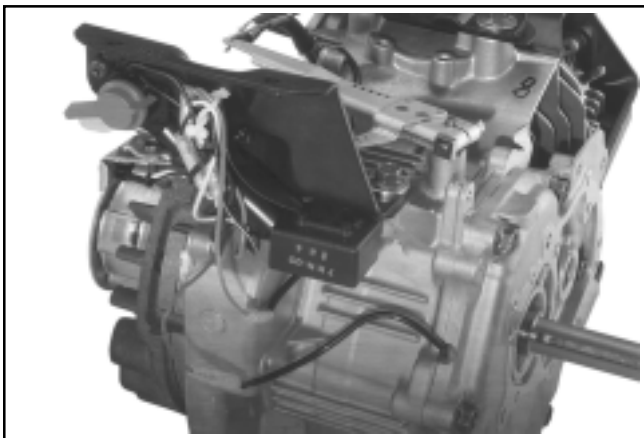
Figure 11-93. CS8.5 (spec. 92xxxx), CS10, CS12. Reconnect Electrical Leads.
