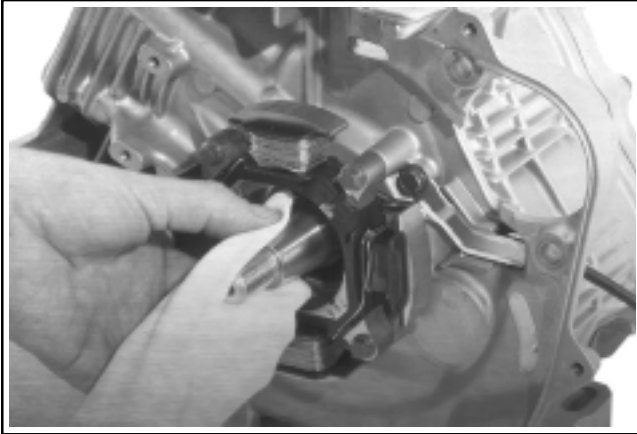
Figure 11-57. Clean and Dry Taper of Crankshaft.
