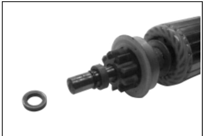
Figure 8-50. Starter Drive and Stop Components.
