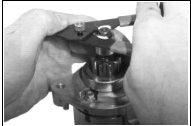
Figure 8-27. Installing Retaining Ring.
