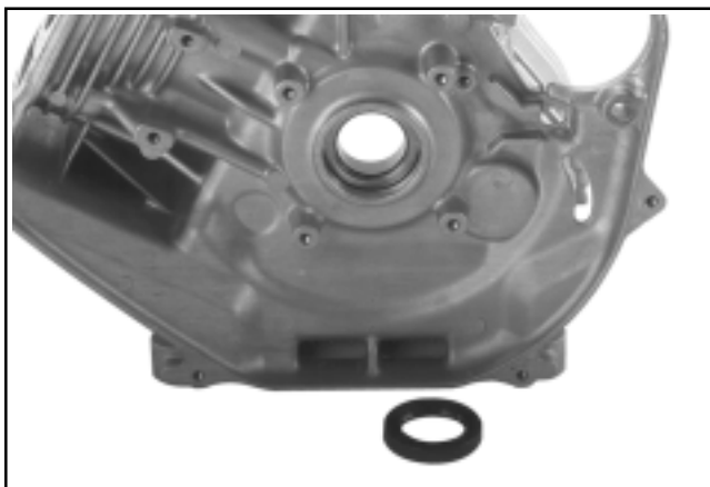
Figure 9-88. Oil Seal Removed.
