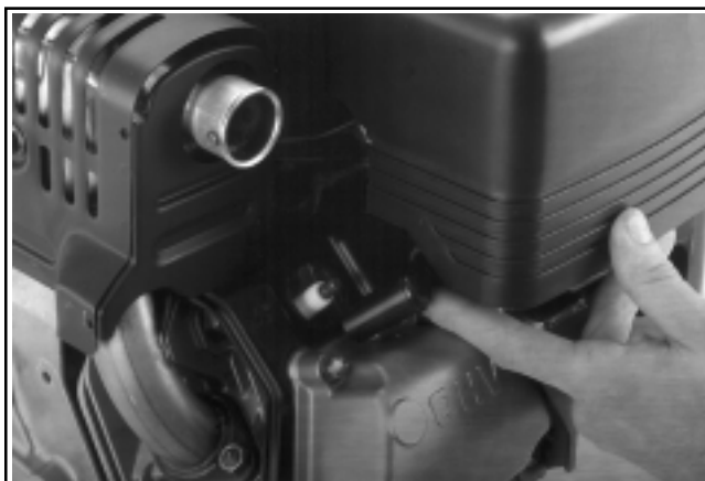
Figure 9-1. Disconnecting Spark Plug Lead.
