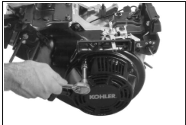
Figure 9-18. Removing Starter Mounting Screws.
