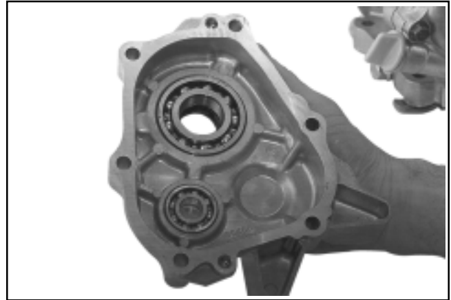
Figure 11-25. CS8.5-12. Installing Bearing.
