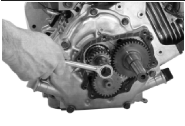
Figure 9-58. Removing Screw from Crankshaft on CS8.5-CS12.
