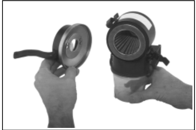
Figure 4-11. Installing Heavy-Duty Cover/Housing.
