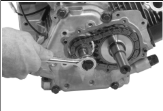
Figure 9-57. Removing Screw from Crankshaft on CS4, CS6.
