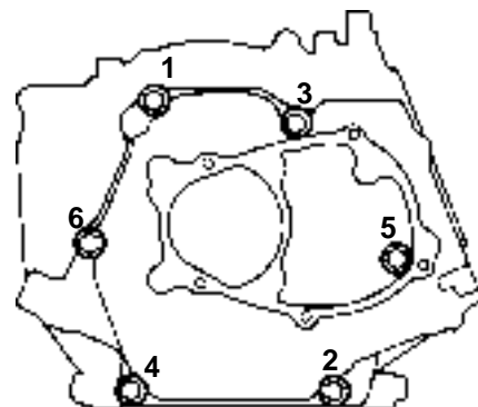
Figure 11-22. CS4, CS6. Closure Plate Torque Sequence.
