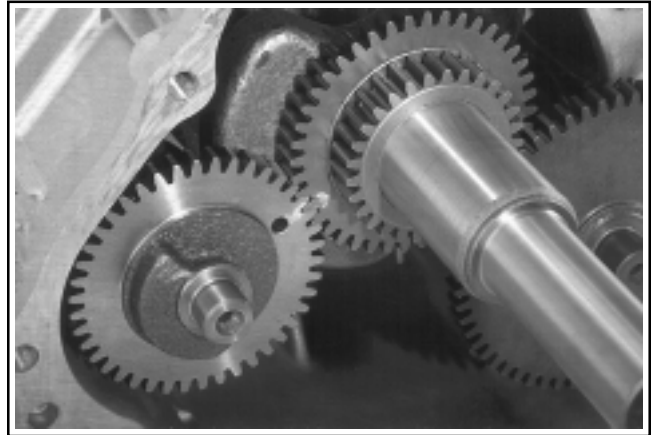
Figure 11-17. CS8.5-12. Aligning Balance Shaft and Crankgear Timing Marks.
