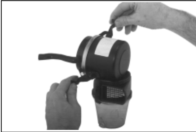
Figure 4-4. Unsnapping Heavy-Duty Latches.
