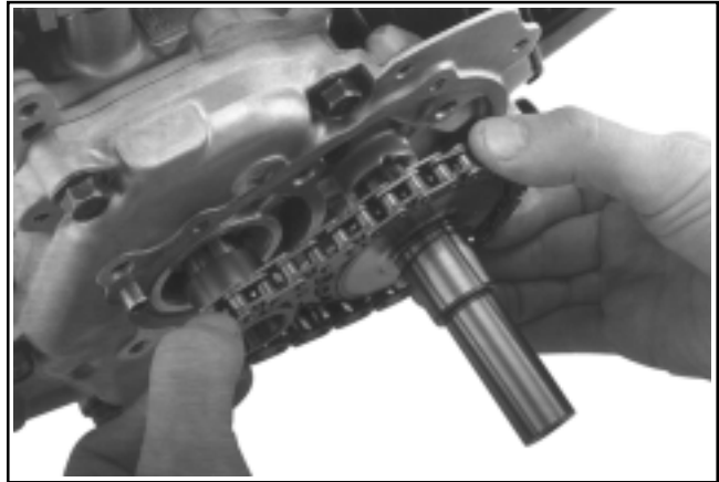
Figure 9-59. Removing Sprockets and Chain on CS4, CS6.
