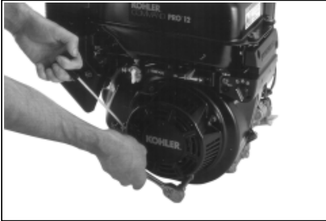
Figure 7-3. Engage Pawls and Tighten Mounting Screws.
