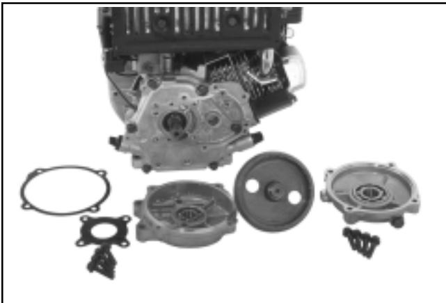
Figure 9-68. CS4, CS6 6:1 Reduction Assembly Components.
