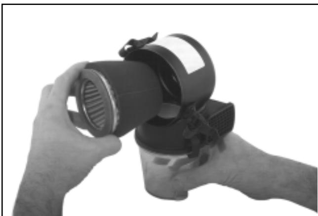
Figure 4-6. Heavy-Duty Element/Precleaner Assembly.
