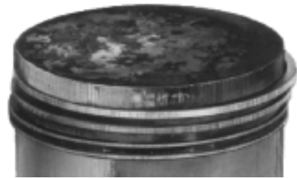
Abrasive Scratched Rings
