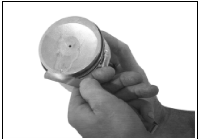
Figure 10-15. Measuring Piston Ring Side Clearance.
