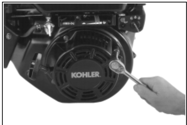
Figure 7-2. Installing Retractable Starter.
