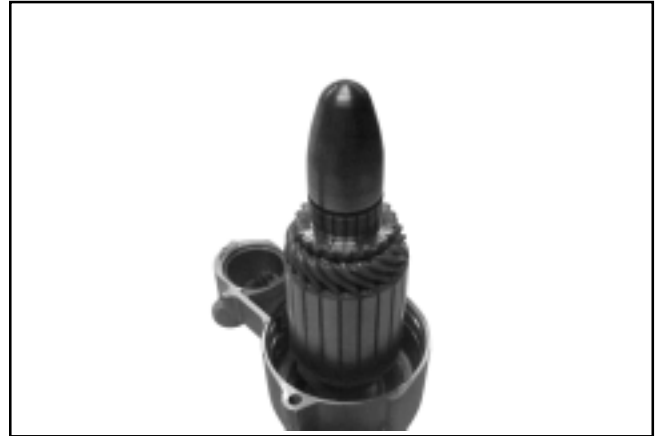
Figure 8-55. Tool on end of Armature.
