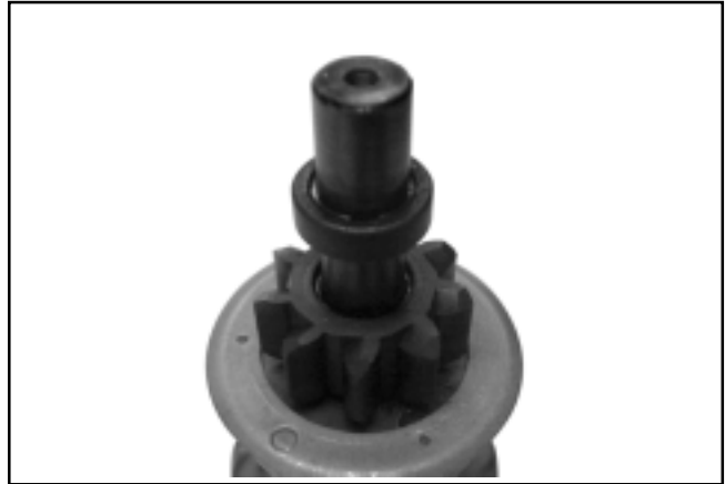
Figure 8-51. Lock Collar around Retaining Ring.
