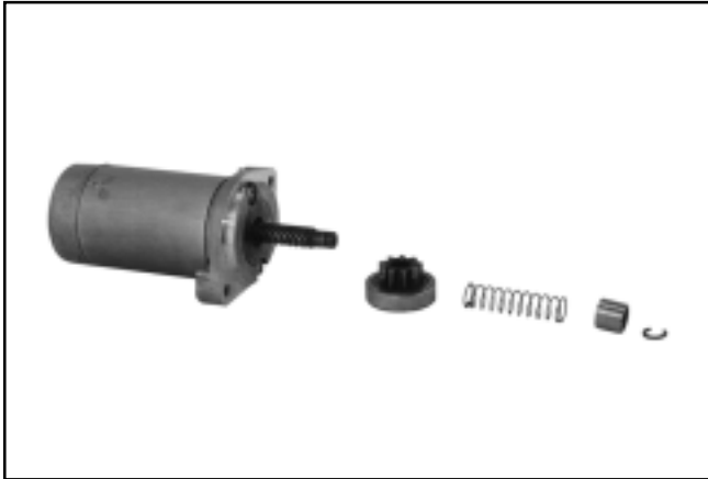
Figure 8-25. Disassembled Drive Components.
