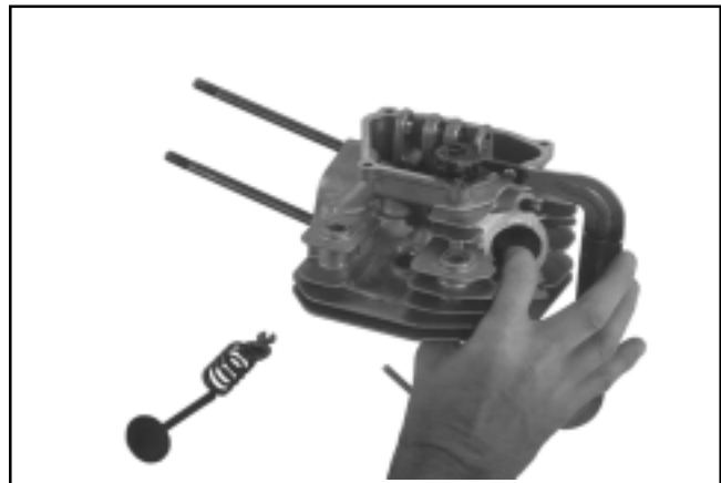
Figure 11-64. Installing Valves Using Valve Spring Compressor.
