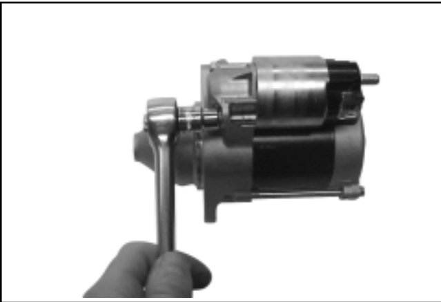
Figure 8-58. Installing Thru Bolts.
