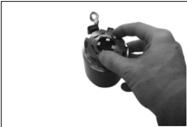
Figure 8-54. Holding Insulator in Place.
