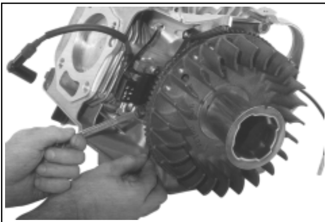
Figure 11-62. CS8.5-12. Setting Air Gap.
