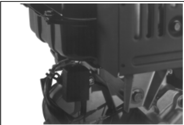
Figure 9-25. CS8.5 (spec. 95xxxx) Ground Lead Location.
