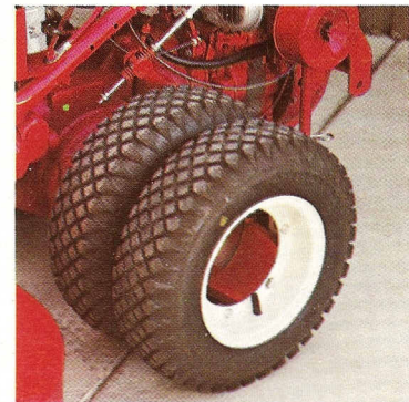
Dual wheels are available as optional equipment and must be used with the Steering Sulky to insure proper stability and traction.
