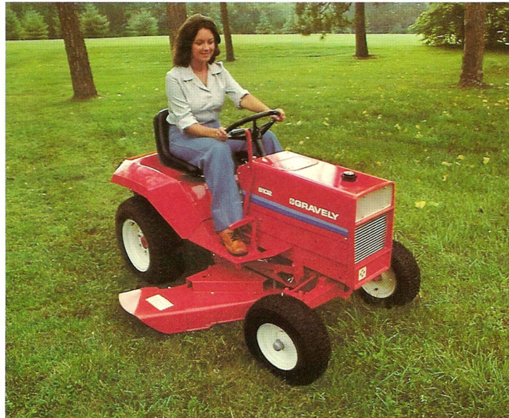
Top: Gravely 8183-T, 18 hp Riding Tractor with 40" Front-Mount Two-Blade Rotary Mower, used with optional Front Drive Kit and Front Adaptor Kit. Bottom: Gravely 8102, 10 hp Riding Tractor with 40" Three-Blade Center-Mount Rotary Mower.
