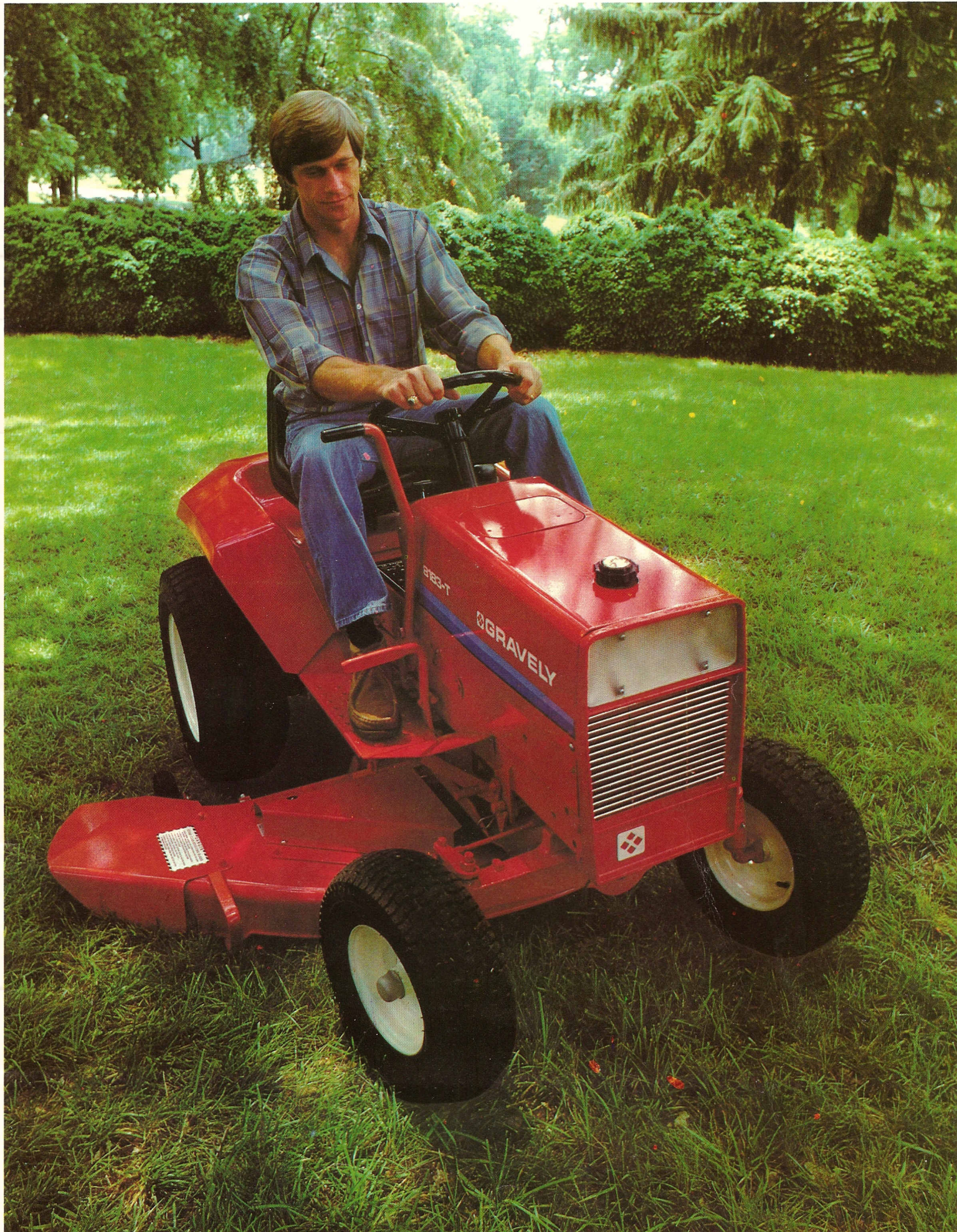
Gravely 8183-T, 18 hp Riding Tractor with 50" Three-Blade Center-Mount Rotary Mower:
