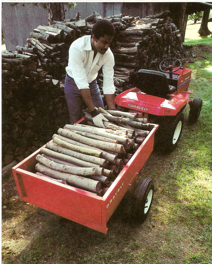
Top: Gravely 8163-T, 16 hp Riding Tractor with all-gear and chain drive Rear Tiller, and optional Front Weight Rack with Weights. Bottom: Gravely 8123, 12 hp Riding Tractor with all-steel Hauling Cart.
