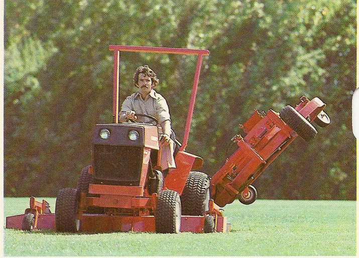
Optional wing lifted and lowered hydraulically with finger tip control.
