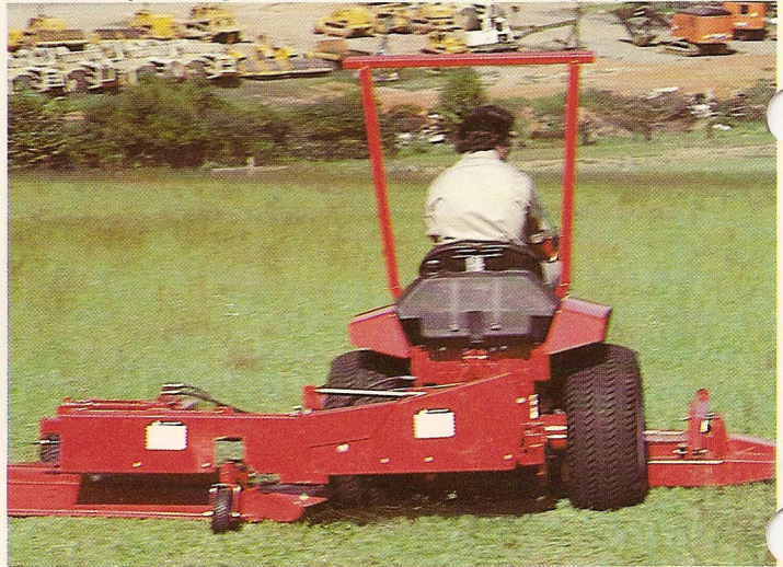
Wing mower power source is line rear PTO.
