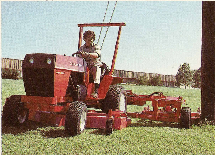
Optional wing cuts within one inch (2.54cm) of poles, fences, trees, shrubs, and other obstacles.
