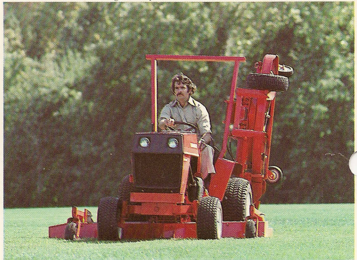
Optional wing folds up when not in use; overall width in transport position 77" (1.96m).
