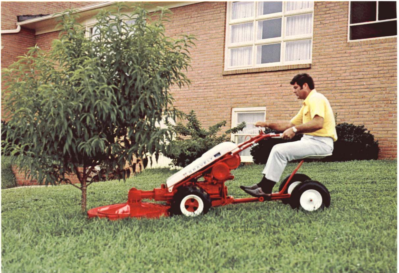
7.6 HP Custom Tractor with 30-Inch Rotary Mower, Optional Chain Guard, and Riding Sulky
