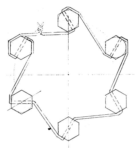
Note position of wire thru the holes tends to tighten the cap screws when tension is put on the wire.
