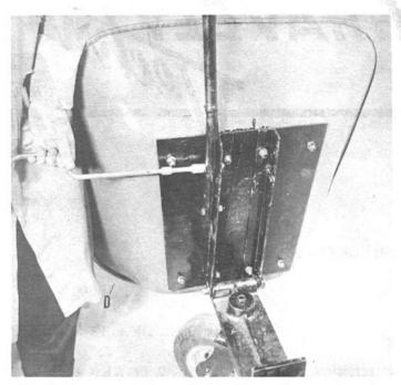
STEP 3. Mount Tray (D) to Tray Support, using eight Bolts and Nuts to secure firmly. Insert Bolts through Tray side and screw Nuts tightly beneath. Attach Dumping Handle in position shown, make sure Bolts are tight.
