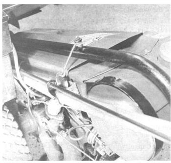
STEP 4. When working on slopes or other rough terrain, you may desire to use the Latch. Attach Bolt and Latch on Dumping Handle-secure Eye on Tractor Handle Bolt. A large and small Spacer is required to attach. You have to bend Eye slightly to work properly.
