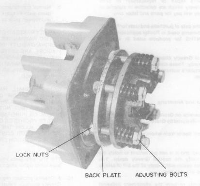
The Attachment Adapter Kit is completely factory assembled and needs only to be bolted to the advance casting of the tractor.
