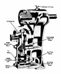
The heart of any sprayer is the pump. The pump used on the Gravely Home'n - garden Sprayer is the nationally famous Myers Du-all Spray pump. This is a double acting, positive displacement pump that delivers ample capacity at all pressures. All working parts are enclosed and fully protected, require a minimum of maintenance.
